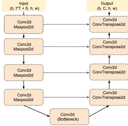
Figure 3.1: Sample U-Net architecture: Left side consists of downsampling blocks and the right side consists of upsampling blocks. The arrows represent the flow of the output. Variables:  $t$  - number of time steps,  $T$  - number of temporal features,  $S$  - number of static features,  $b$  - batch size,  $h$  - height,  $w$  - width
