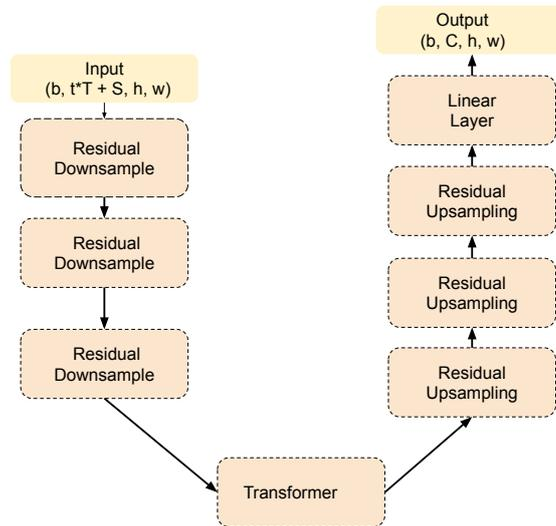
Figure 3.4: PT-Net Architecture: The input batch is encoded by the down-sampling layers, accumulated by the attention modules, and then upsampled into the output. Figure notations are the same as in Figure 3.2.
