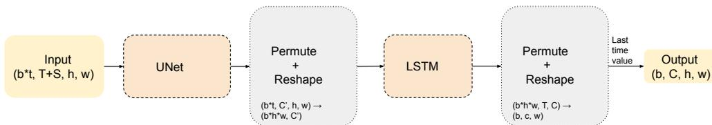
Figure 3.2: UNet-LSTM Architecture: Each batch is first fed into the U=Net component and then reshaped before being passed into the LSTM layer.  $b$ : batch size,  $h$ : height,  $C'$ : number of output channels from the U-Net component,  $C$ : number of output channels—one for each class
